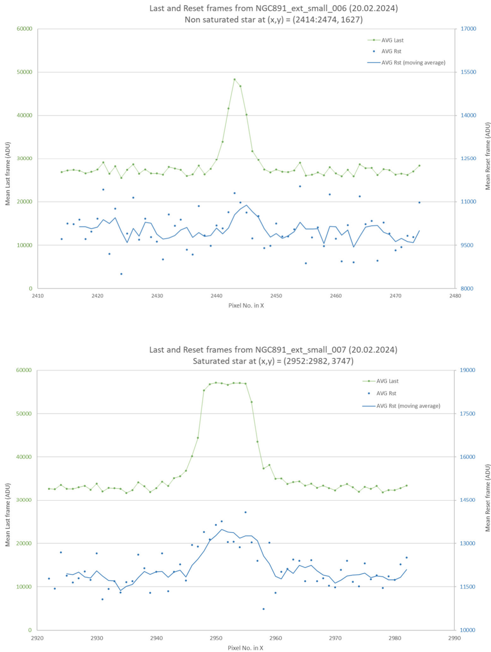
Figure 3. Reset frame behavior (1x reset) of pixels corresponding to the position of bright stars. Top: non-saturated star. Bottom: saturated star
