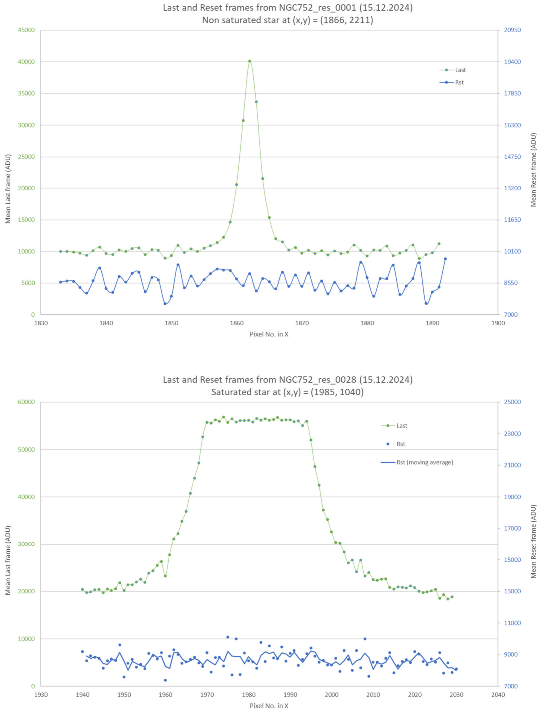
Figure 5. Reset frame behavior (10x resets) of pixels corresponding to the position of bright stars. Top: non-saturated star. Bottom: saturated star
