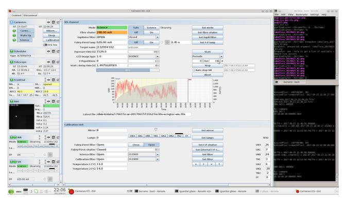
In GTO mode, Target name and Exposure time in NIR and VIS tabs is filled automatically. In non-GTO mode, fill Target name and Exposure time in NIR and VIS tabs. For the moment, Target name in NIR and VIS must be identical.
