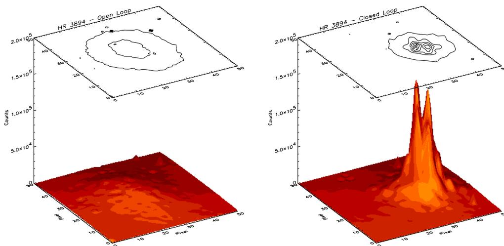
**Figure 4:** A near infrared image of the 0.24'' binary  $\phi$  Ursa Majoris (HR 3894,  $m_V = 4.6$ ) observed through clouds in 1.7'' seeing on March 1, 1997. The observing wavelength was 2.2 $\mu$ m. 20 Zernike modes were corrected with a frame rate of 900 Hz. This is a raw image without any image processing adding up single images to a total exposure time of 50sec. The two components are clearly resolved.
