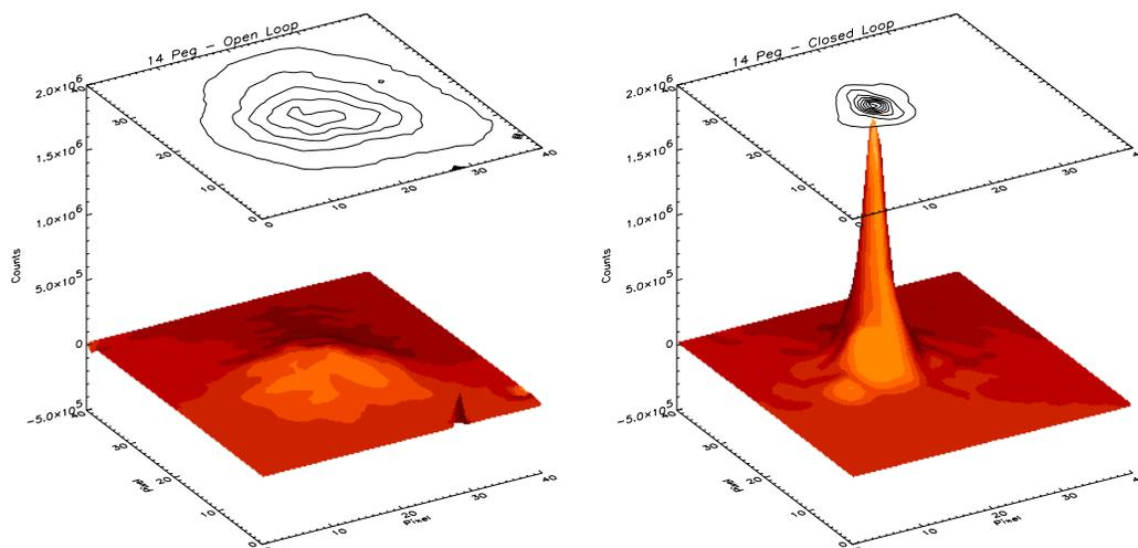
**Figure 6:** Uncorrected and corrected images of 14 Peg ( $m_V = 5.04$ ) at  $2.2\mu\text{m}$  taken on July 21, 1997. Correcting 17 Zernike modes with a loop frequency of 100Hz the Strehl ratio is improved from 2.4% to 20% in  $0.85''$  seeing. No image processing was applied.
