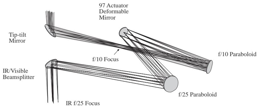
**Figure 1:** The main optical elements of the optical system of ALFA.
