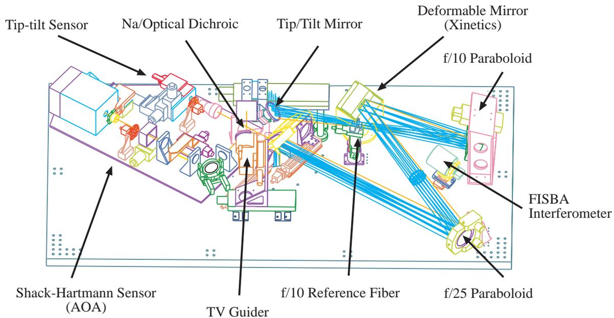
**Figure 2:** The ALFA breadboard with all opto-mechanical elements.
