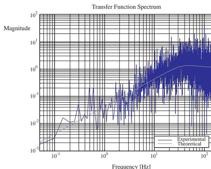
**Figure 5:** The measured and the theoretical transfer function of the closed loop system for the Zernike mode  $J = 4$  (focus). The measured transfer function is the quotient of the uncorrected and the corrected spectrum. The theoretical function is calculated using the parameters of the control loop.
